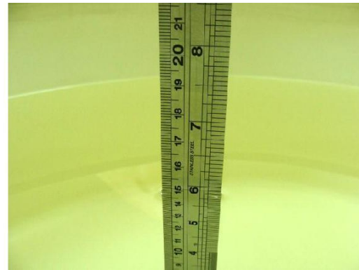
Fig 6.2 Photo of Liquid Height for Body SAR
